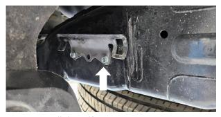
Fig. 20: Install the self tapping screw (passenger side shown).
