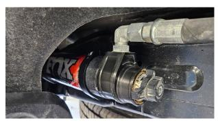
Fig. 23: Mount the reservoir to the bracket (driver side shown).
