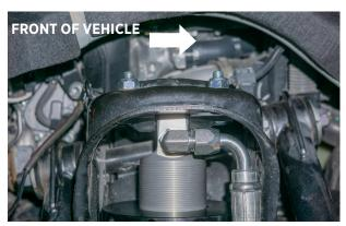
Fig. 9: The hose fitting faces outboard.
