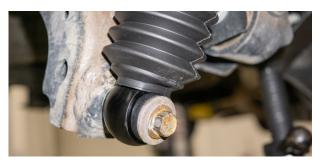
Fig. 22: Install the lower shock bolt (passenger side shown).
