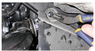
Fig. 4: Remove sway bar bracket.
