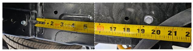
Fig. 19: Drill two pilot holes.
