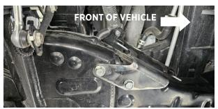
Fig. 5: Install the reservoir bracket assembly.
