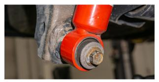
Fig. 18: Remove lower shock mount bolt.
