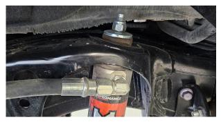
Fig. 21: Install the stem top nut (passenger side shown).
