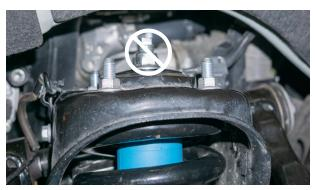
Fig. 7: Remove the four top hat nuts. Do NOT remove the center nut.
